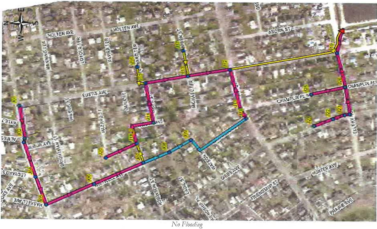
Figure 21. Simulated Peak Flooding Depths under Alternative 2: Increase Pipe Sizes and Watson Street Connection (August 15, 2012 Storm Event)
