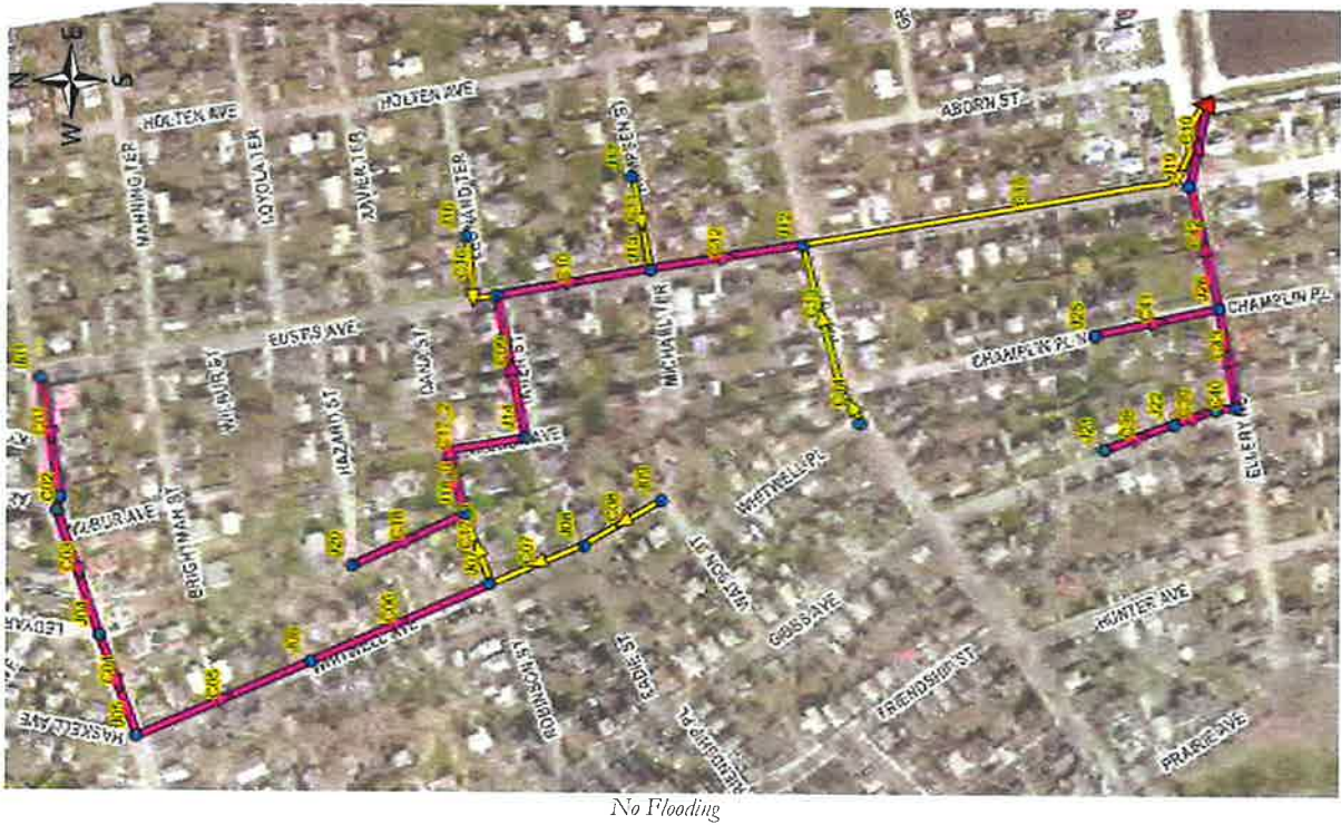
Figure 16. Simulated Peak Flooding Depths under Alternative 1: Increase Pipe Sizes (August 2012 Storm Event)
