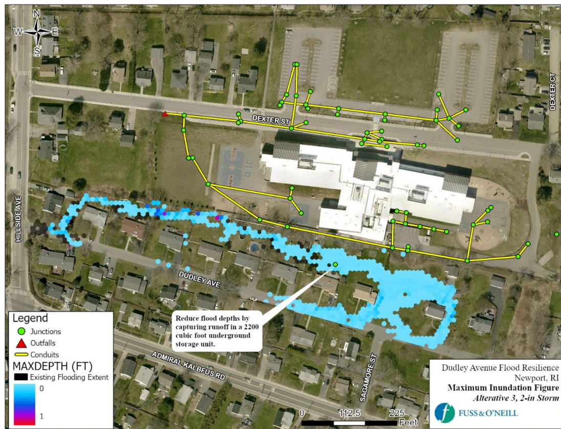
Figure 23. Simulated Peak Flooding Depths under Alternative 3 (2-inch Storm Event)
