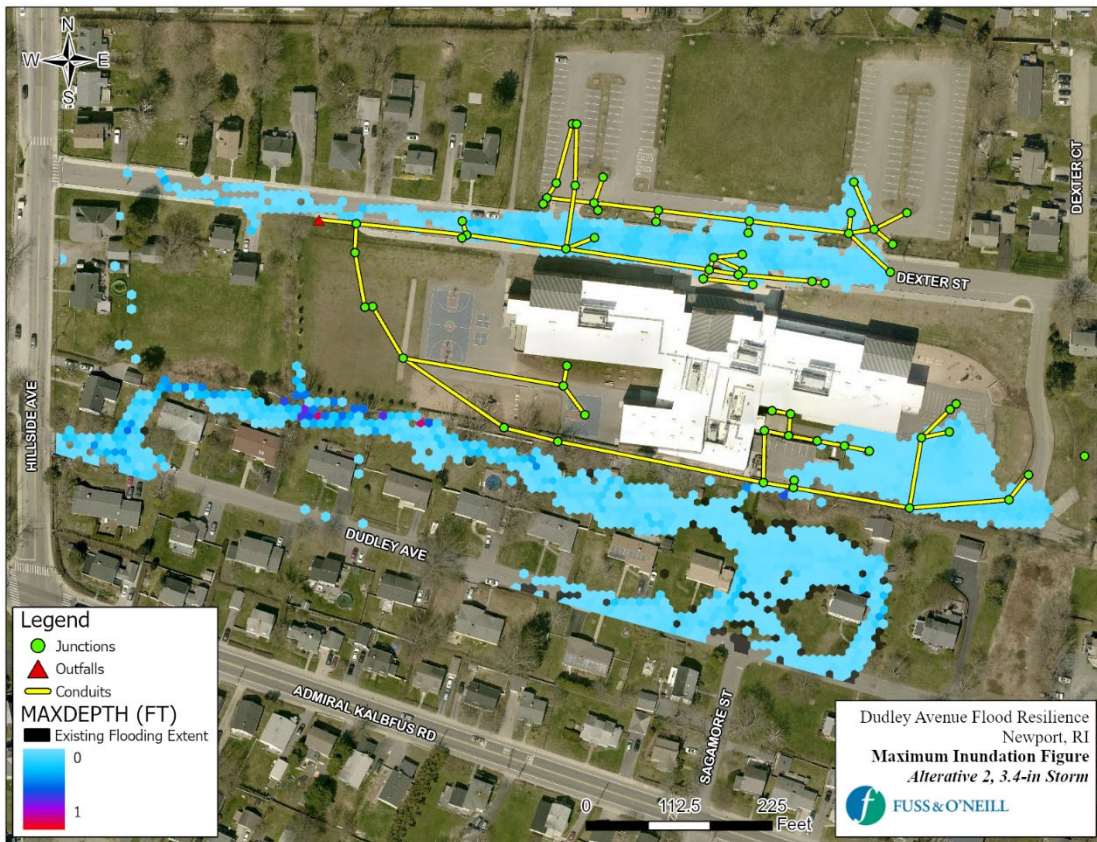
Figure 20. Simulated Peak Flooding Depths under Alternative 2 (2-Year Storm Event)
