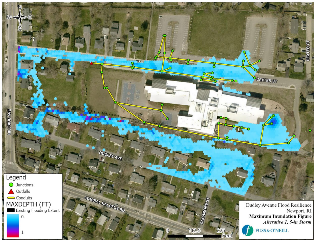
Figure 17. Simulated Peak Flooding Depths under Alternative 1 (10-Year Storm Event)
