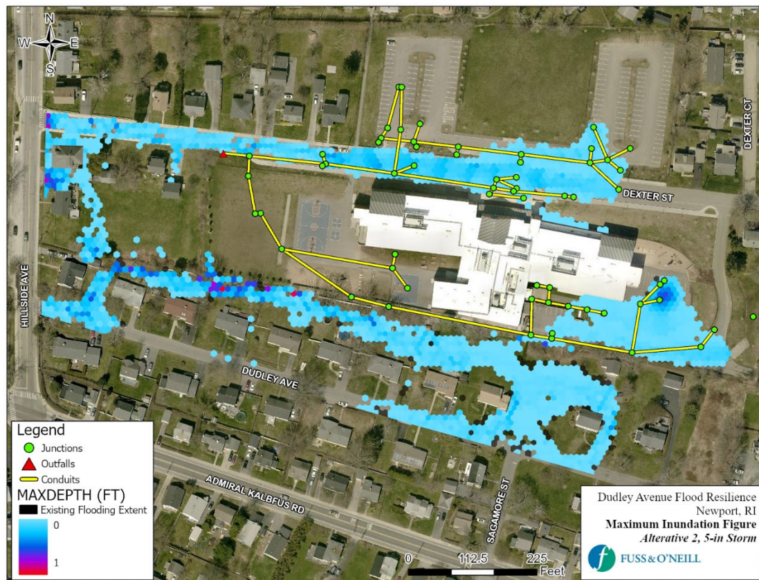
Figure 21. Simulated Peak Flooding Depths under Alternative 2 (10-Year Storm Event)
