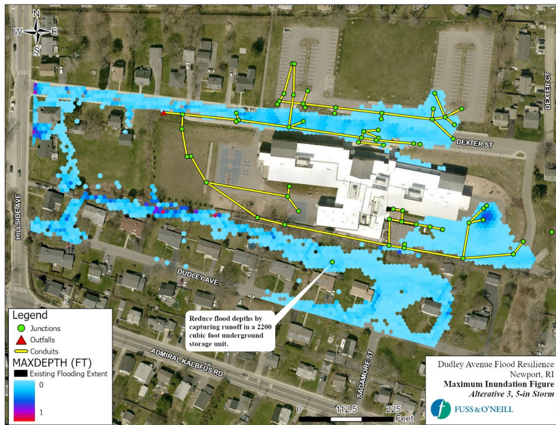
Figure 25. Simulated Peak Flooding Depths under Alternative 3 (10-Year Storm Event)
