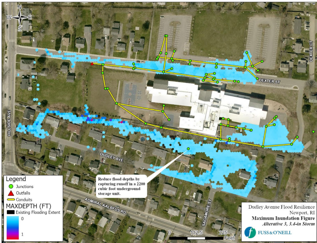
Figure 24. Simulated Peak Flooding Depths under Alternative 3 (2-Year Storm Event)
