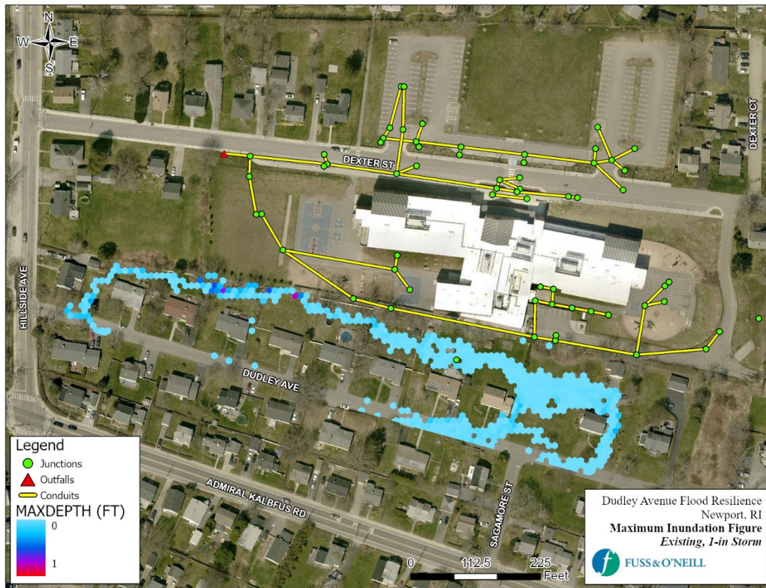
Figure 9. Simulated Peak Flooding Depths under Existing Conditions (1-inch Storm Event)
