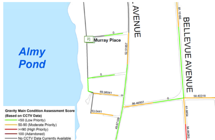
Pipe Condition Scores from CCTV Inspections
