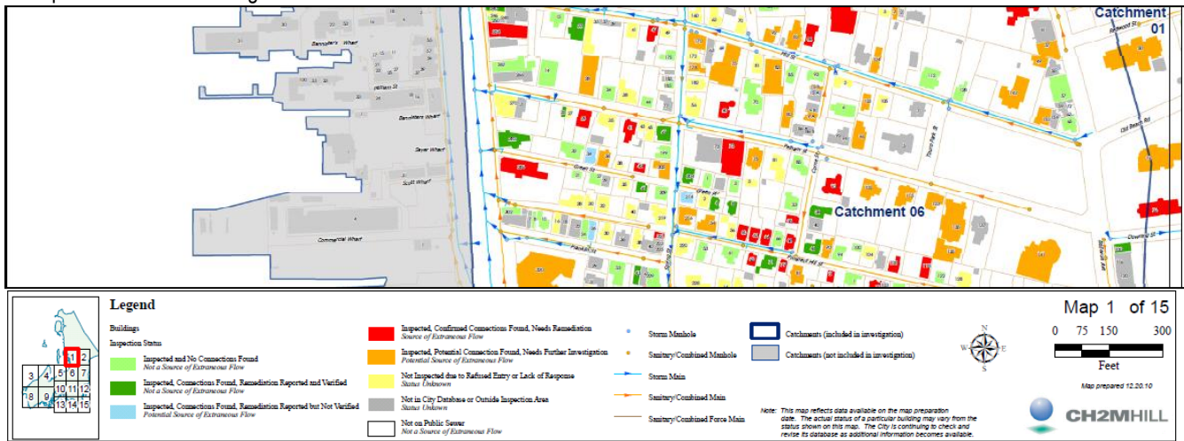
FIGURE 4 Example of Private I/I Investigation Results
