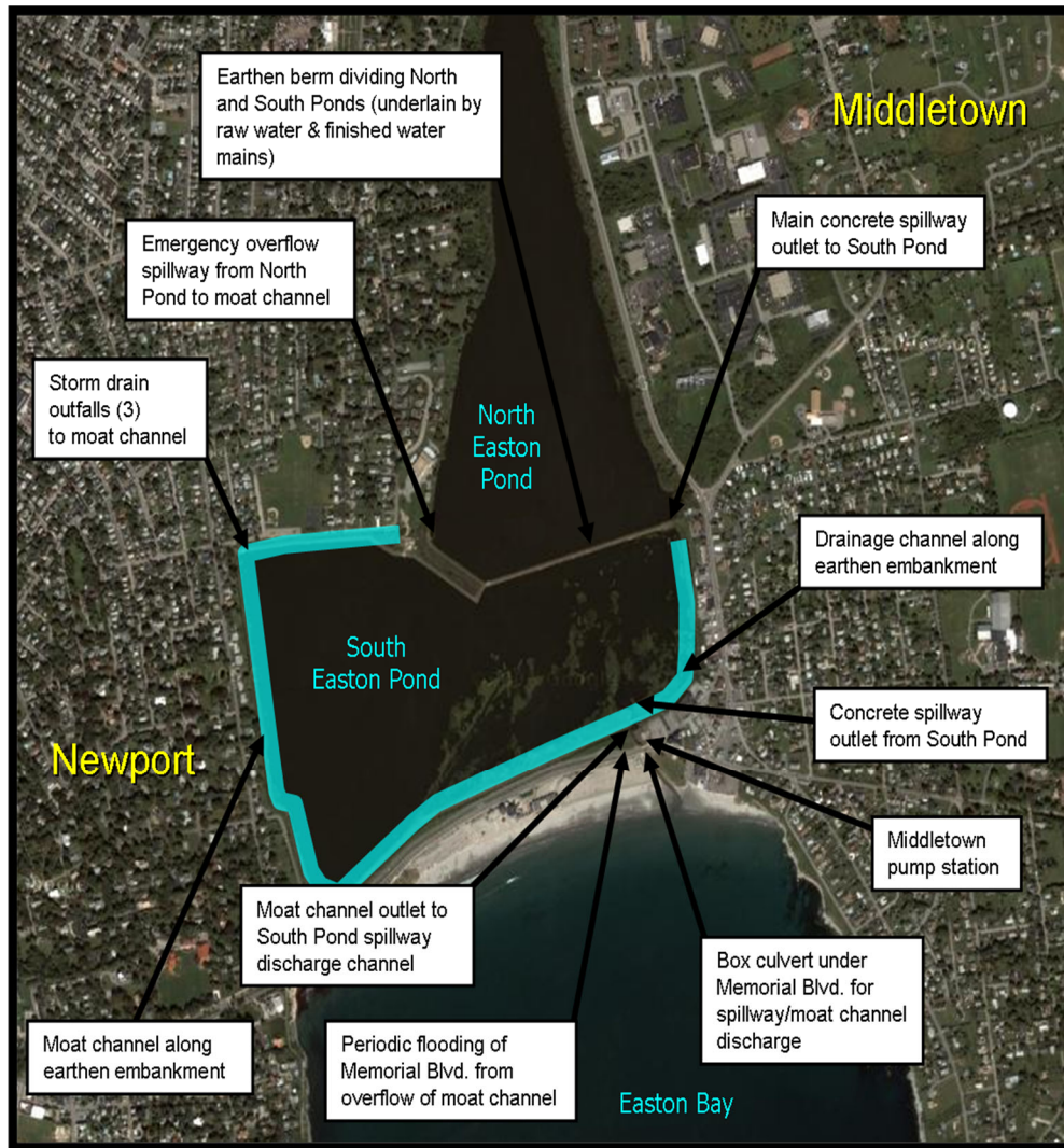
Figure 25 - Hydraulic Connectivity Plan between North Easton Pond, South Easton Pond, and Easton Bay
