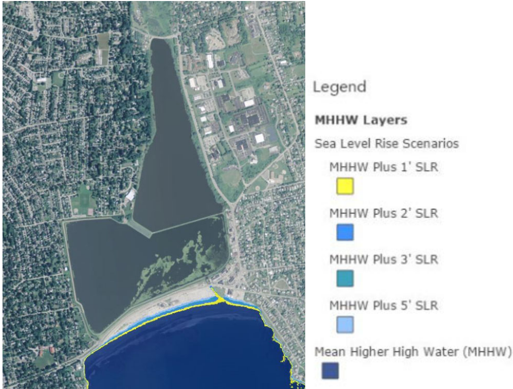
Figure 13 – RICRMC Default Individual Inundation Layers for Projected Sea Level Rise Map for Easton Pond
