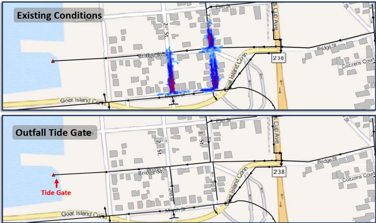
Figure B-7. Bridge Street Outfall Tide Gates – King Tide Comparison between existing conditions and outfall tide gates for the 10/27/2011 King Tide of 5.9 ft (MLLW), no rain
