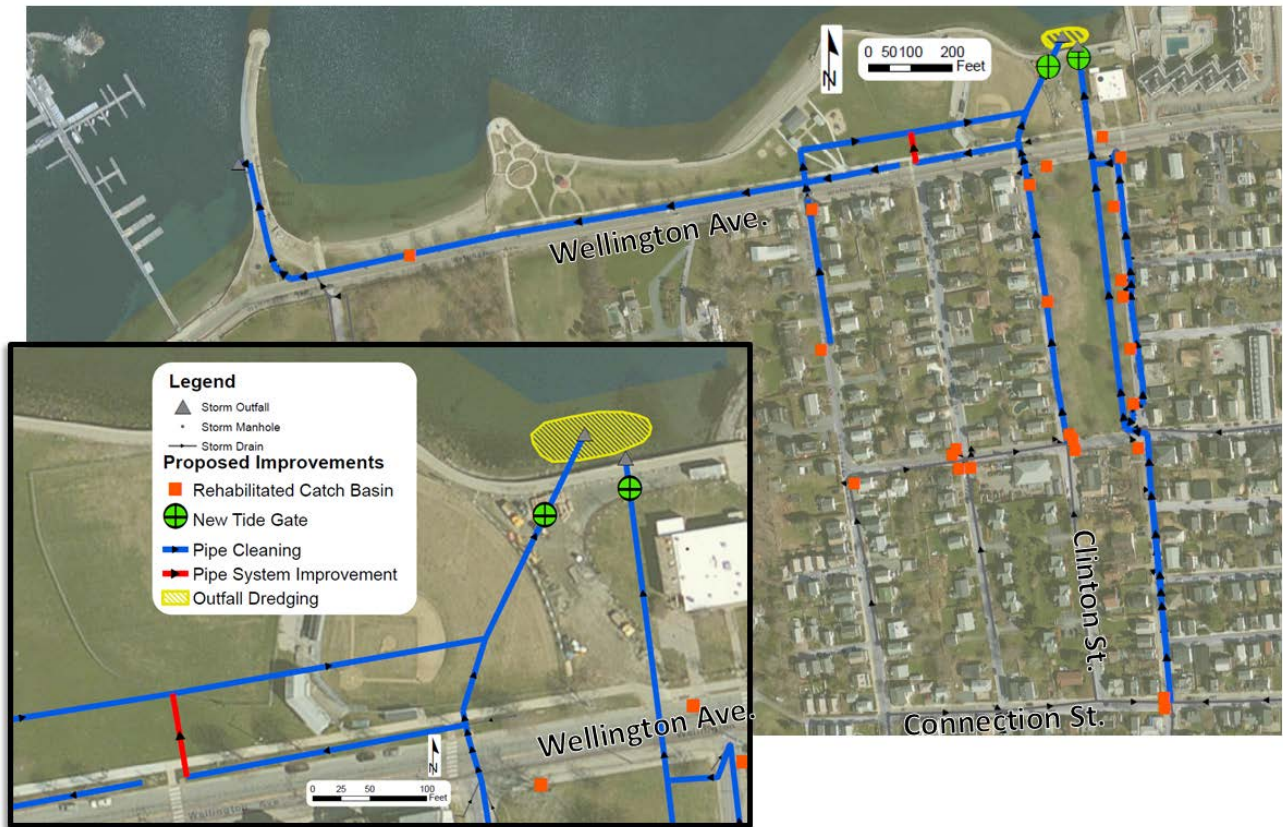
Figure 6-1. Conceptual Layout of the Short-term controls in the Wellington Avenue Study Area
