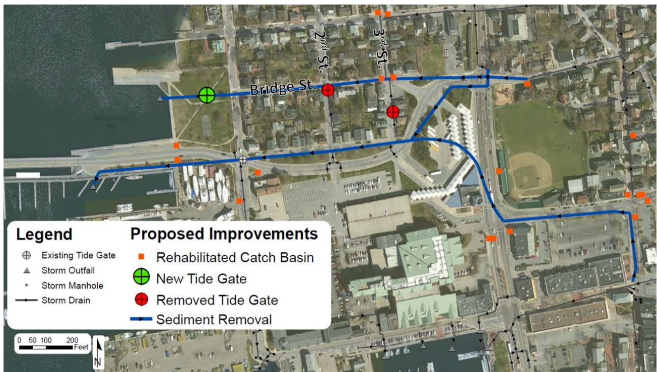
Figure 6-4. Conceptual Layout of the Short-term controls in the Bridge Street Study Area
