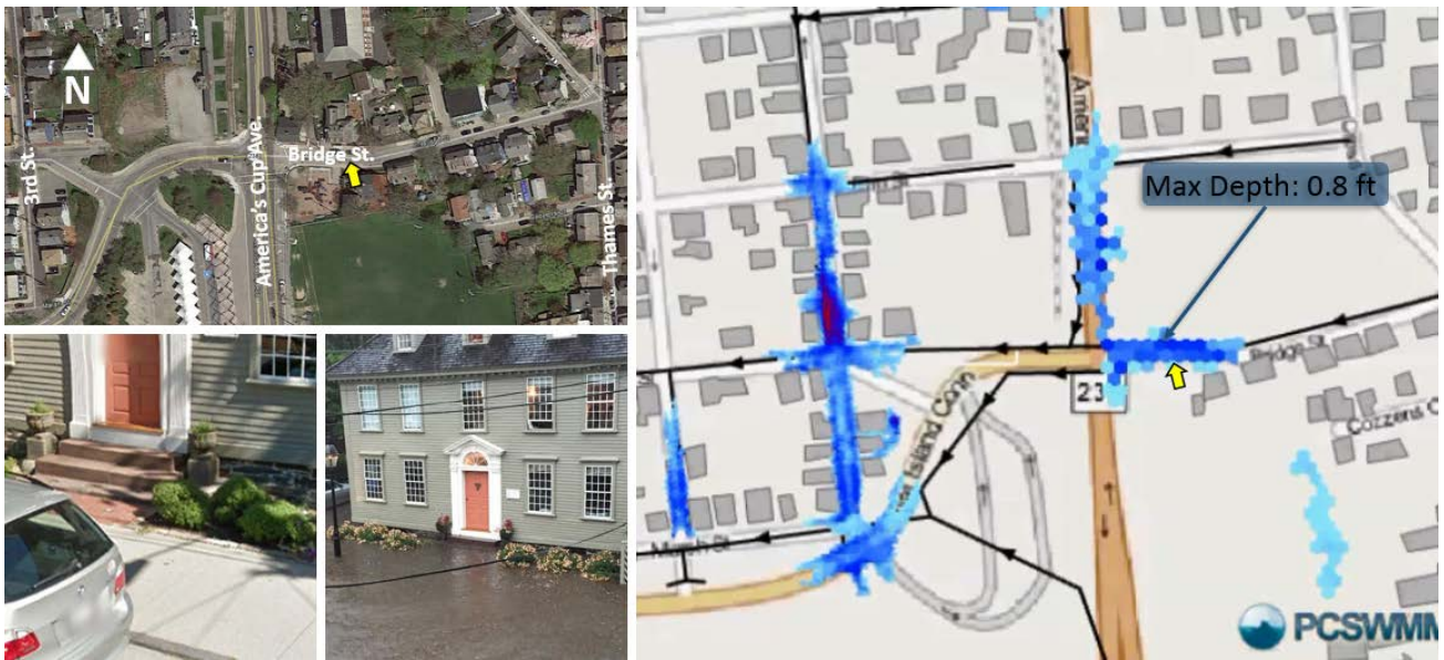
Figure 3-3. Bridge Street Wet Weather Flooding Calibration Event This was a 1.2 inch rainfall event occurring at a high tide of 4.3 feet (MLLW) on July 1, 2015
