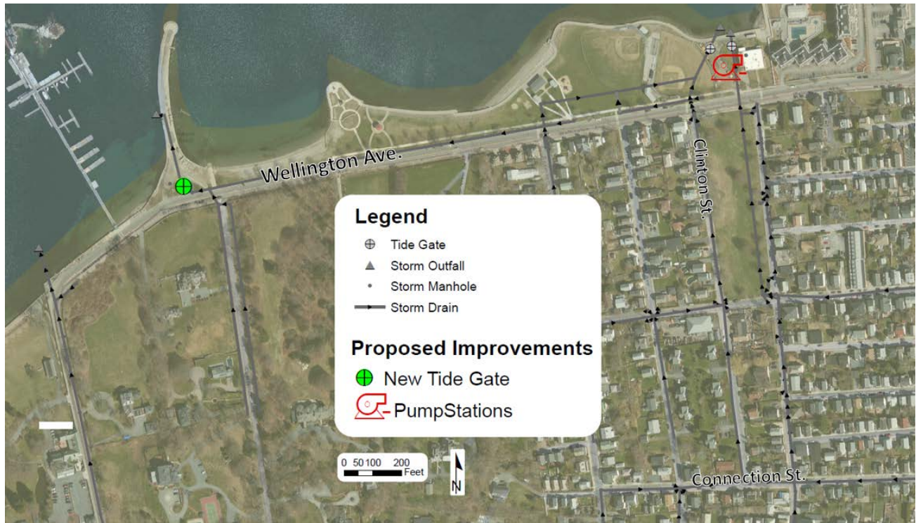
Figure 6-3. Conceptual Layout of the Long-term controls in the Wellington Avenue Study Area
