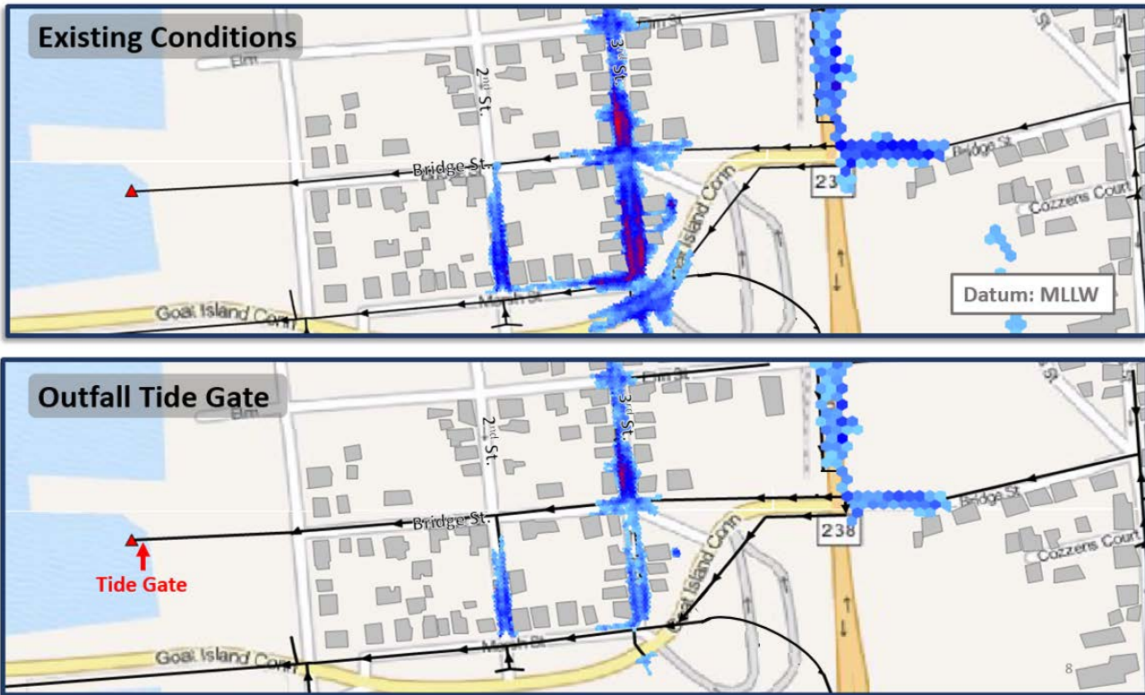
Figure B-7. Bridge Street Outfall Tide Gates – King Tide Comparison between existing conditions and outfall tide gates for the 10/27/2011 King Tide of 5.9 ft (MLLW), no rain
