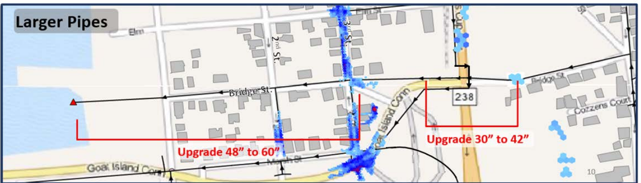
Figure B-10. Bridge Street Larger Pipes – Rain at High Tide Comparison between existing conditions and larger pipes for the 7/1/2015 rain event of 1.2 in at high tide of 4.3 ft (MLLW)
