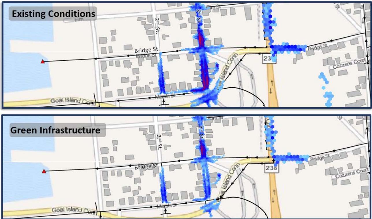
Figure B-11. Bridge Street Green Infrastructure – Rain at High Tide Comparison between existing conditions and green infrastructure for the 7/1/2015 rain event of 1.2 in at high tide of 4.3 ft (MLLW)
