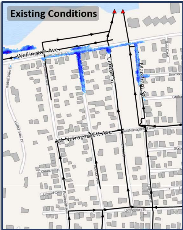
Figure B-3. Wellington Avenue Pipe Sediment Removal – Rain at Low Tide Comparison between existing conditions and pipe sediment removal for the 7/1/2015 rain event of 1.2 in at a theoretical low tide
