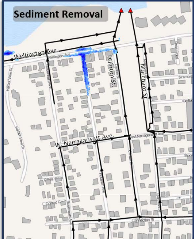
Figure B-3. Wellington Avenue Pipe Sediment Removal – Rain at Low Tide Comparison between existing conditions and pipe sediment removal for the 7/1/2015 rain event of 1.2 in at a theoretical low tide
