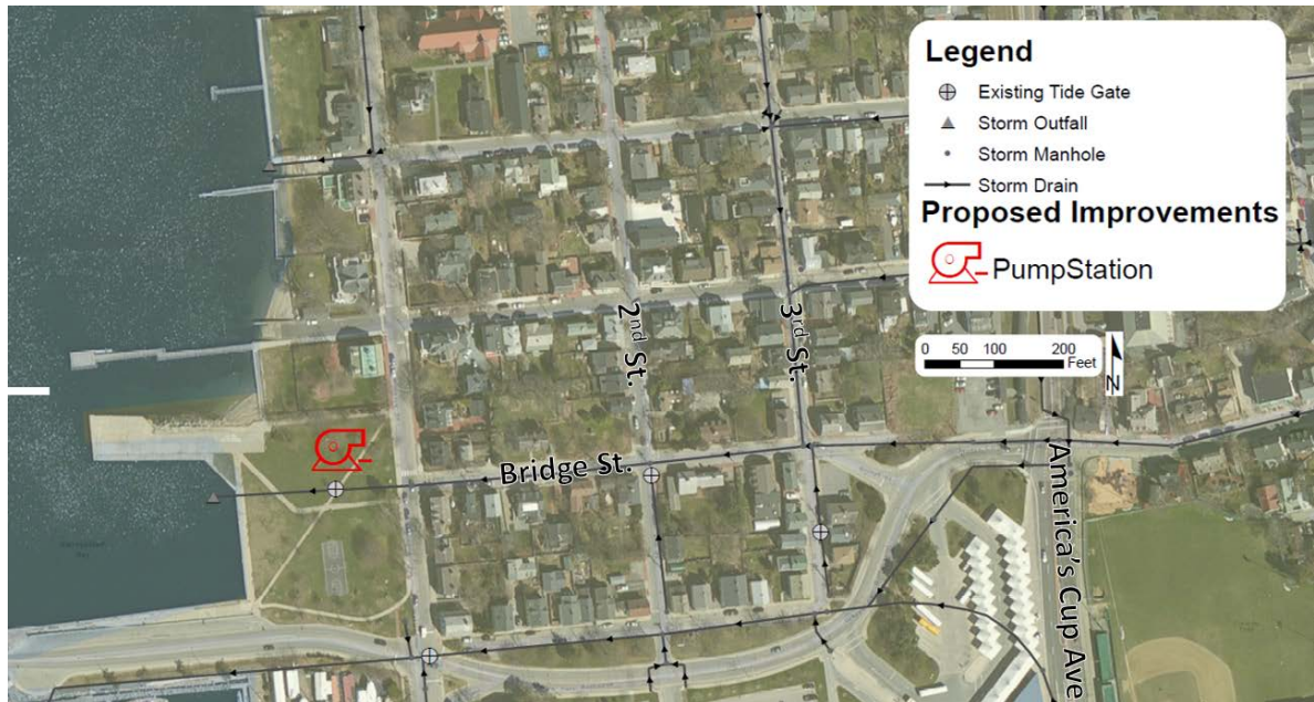
Figure 6-6. Conceptual Layout of the Long-term controls in the Bridge Street Study Area
