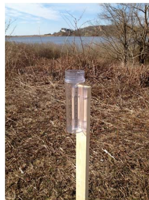
One of two rainfall gauges used during stormwater sampling rounds
