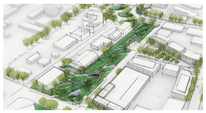
Water management area buffering the Mixed-use Village Core from the. Maker area. While creating more green open space, this area can improve the resiliency of the North End area by absorving and retaining excess water during intense rain events.
