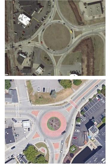
The image at top shows the existing rotary at Admiral Kalbfus Road and JT Connell Highway. The rotary is hostile to pedestrians and out of scale with many surrounding land uses. The bottom image depicts an example alternative design for handling similar traffic patterns, creating a safer and more pedestrian-friendly intersection.
