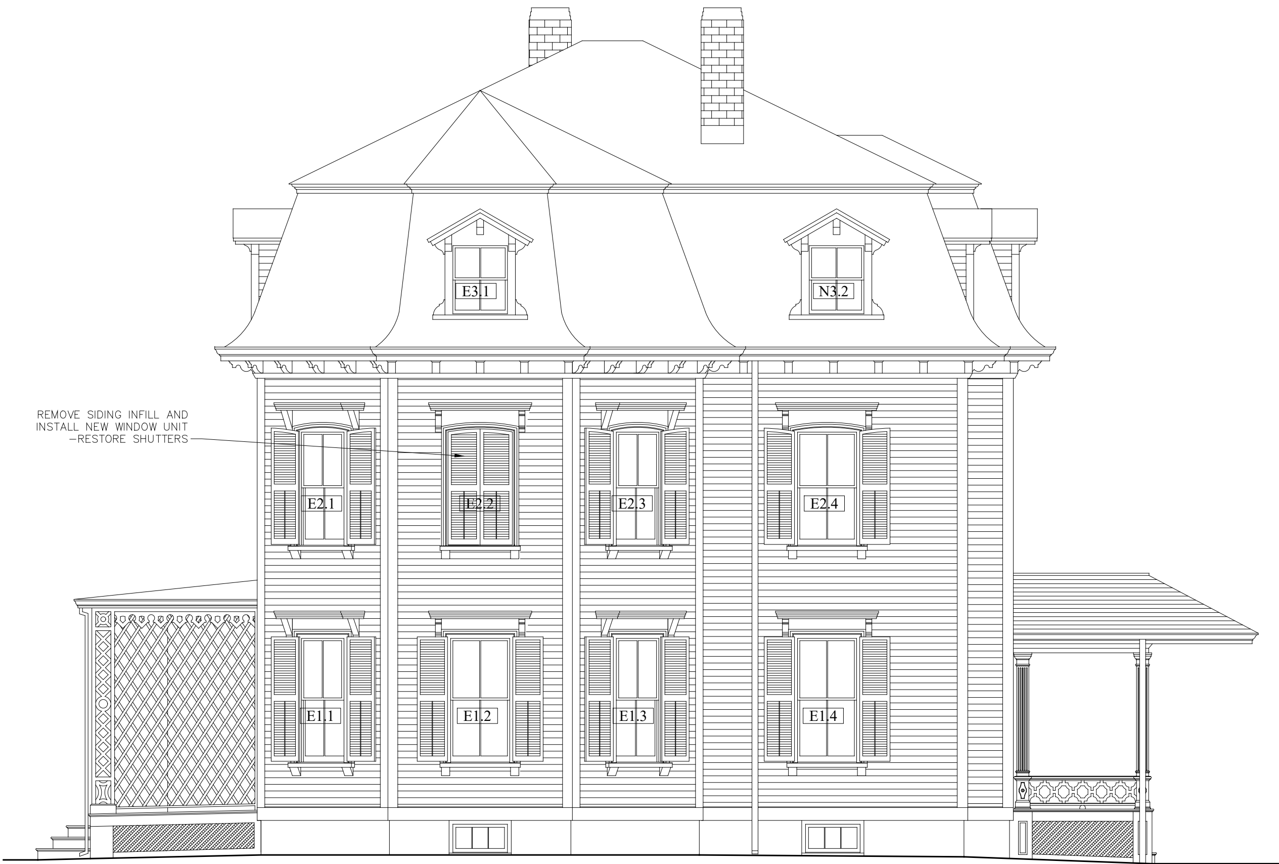
1 A1 EXISTING EAST ELEVATION SCALE: 3/16" = 1'-0"
