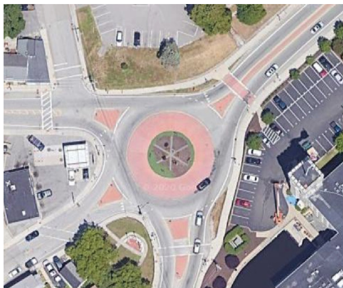
The image at top shows the existing rotary at Admiral Kalbfus Road and JT Connell Highway. The rotary is hostile to pedestrians and out of scale with many surrounding land uses. The bottom image depicts an example alternative design for handling similar traffic patterns, creating a safer and more pedestrian-friendly intersection.
