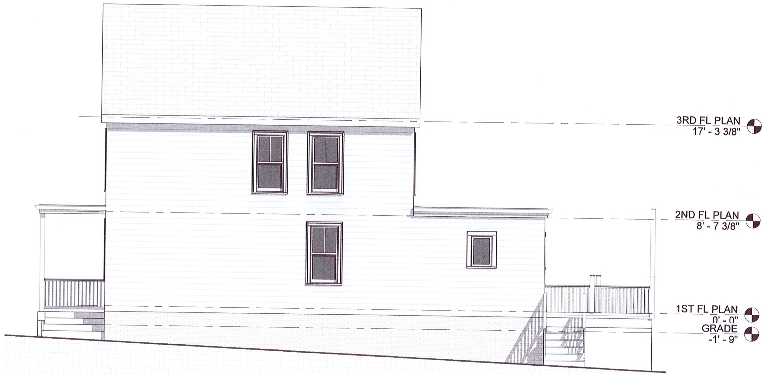
① SOUTH ELEVATION EXISTING 3/16" = 1'-0"
