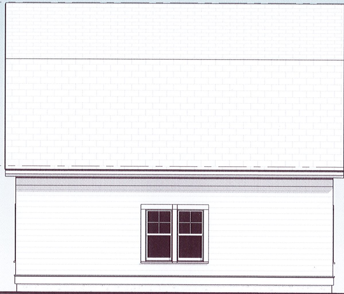
① REAR ELEVATION (NORTH) 3/16" = 1'-0"
