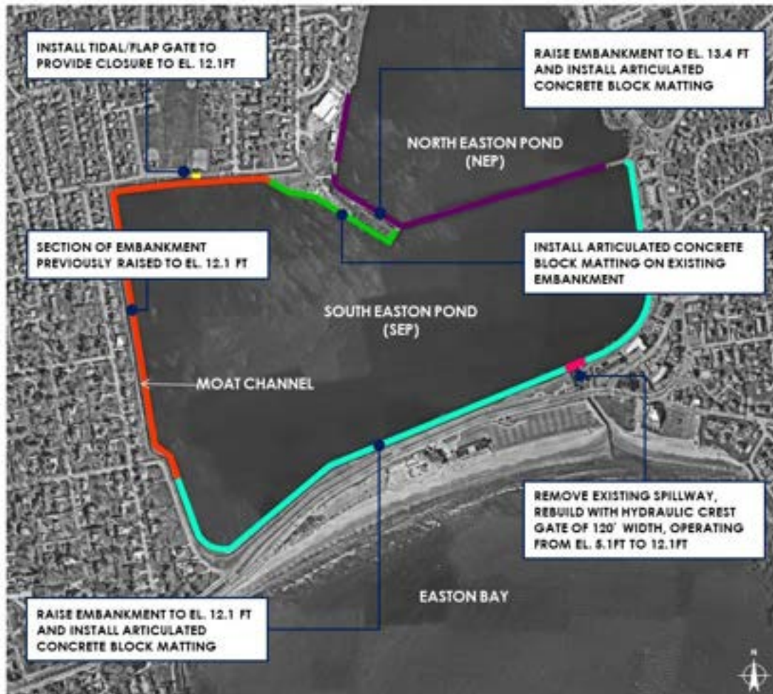
Figure 4: Recommended improvements to NEPD and SEPD.
