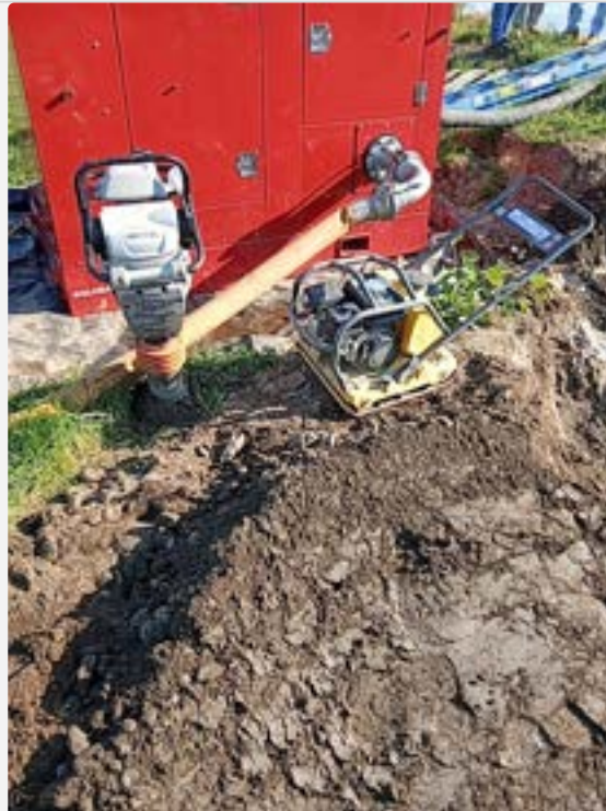
"Compaction Equipment": The Wacker Neuson 1550A vibratory plate compactor & the Mikasa MTX-60 bouncing compactor.
