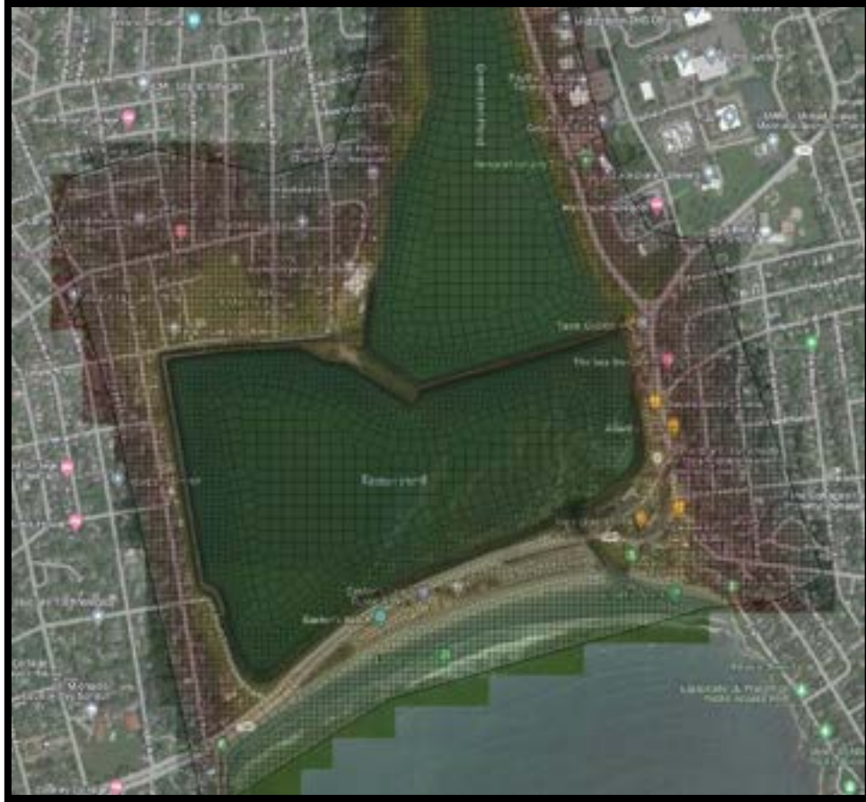
Figure 6: A 2-dimensional cell mesh developed for hydraulic modeling
